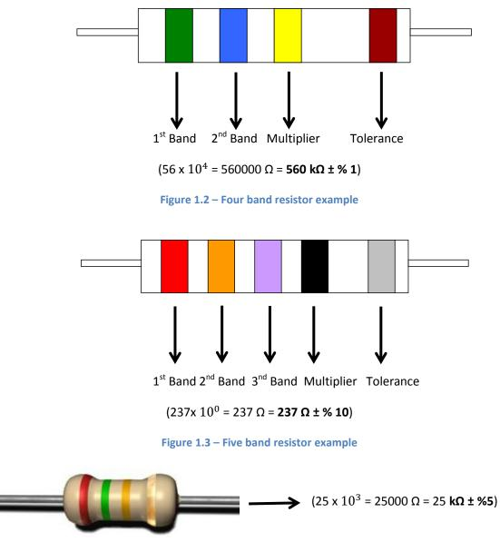
Figure 1.4 – Example resistor and its value
