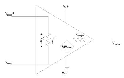
Figure 10.2– Ideal equivalent circuit of OP-AMP
