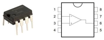
Figure 10.4– LM 741 and internal structure
