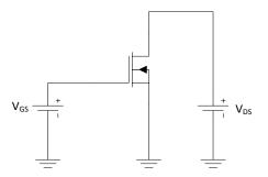
Figure 9.2 – V<sub>GS</sub> and V<sub>DS</sub> connections
