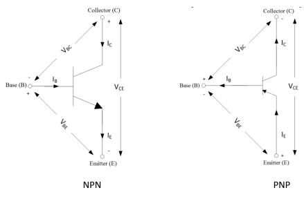
Figure 7.1 – NPN and PNP transistors
