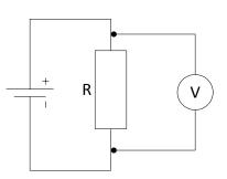
Figure 1 – Voltmeter is connected in parallel
