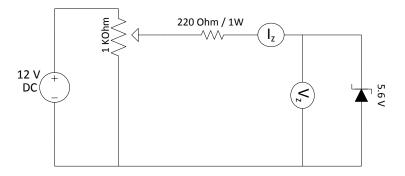
Figure 6.4– Reverse biased circuit
