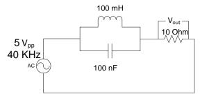
Figure 3.8 – Parallel RLC circuit schematic
