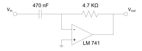
Figure 11.3– Differentiator circuit
