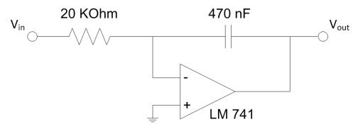
Figure 11.4 – Integrator circuit
