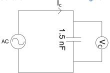
Figure 2.8 – Capacitor in AC circuit
