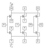
Figure 9.5 – CD4007 pin connections
