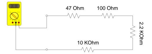
Figure 1.5 – Resistors connected in series experiment schematic
