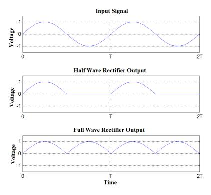
Figure 5.1 – Output signals of half wave and full wave rectifiers
