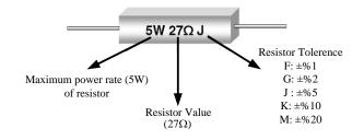
Figure 1.1 – Resistor value coding by digits
