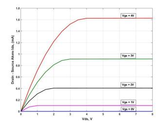
Figure 9.3 – I<sub>DS</sub> / V<sub>DS</sub> graph
