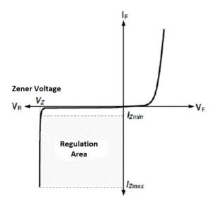
Figure 6.2 – Zener diode characteristic curve
