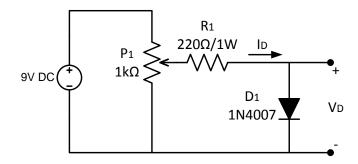
Figure 4.2 – Forward bias circuit
