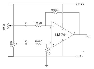
Figure 10.8– Difference amplifier circuit
