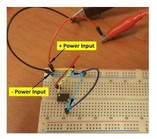
Figure 6 – Integrated circuit placement example
