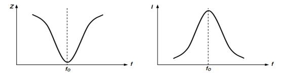
Figure 3.5 – Impedance-frequency and current-frequency relations of serial RLC circuits
