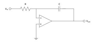
Figure 11.2 – Integrator circuit
