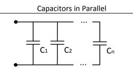
The voltage of each capacitor is equal when the capacitors connected in parallel.  $V_1 = V_2 = \cdots = V_n$
