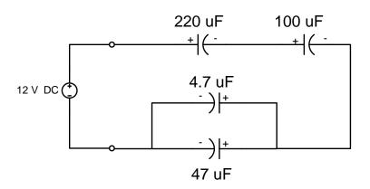
Figure 1.8 – Capacitors connected in series and parallel
