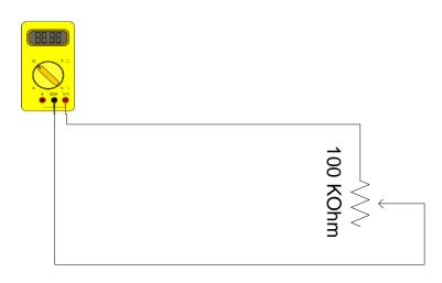
Figure 1.6 – Potentiometer experiment schematic
