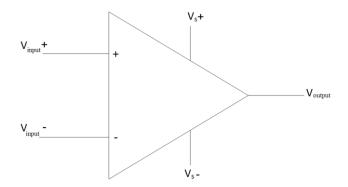
Figure 10.1– OP-AMP symbol and input/output terminals
