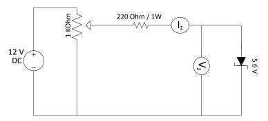
Figure 6.3 – Forward biased circuit
