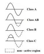
Figure 8.1 – Classification of amplifiers according to their transmission status
