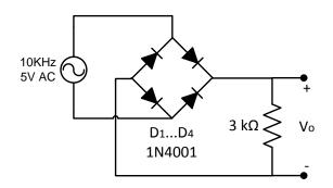
Figure 5.4 – Unfiltered full wave rectifier
