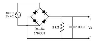
Figure 5.5 – Filtered full wave rectifier
