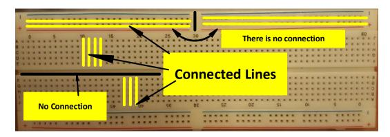
Figure 4 – Breadboard rails and connected holes
