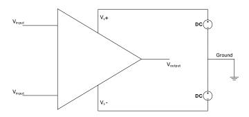
Figure 10.3– OP-AMP supply circuit
