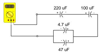
Figure 1.7 – Capacitor circuit connected in series and parallel, equivalent capacitor calculation
