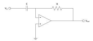
Figure 11.1– Differentiator circuit
