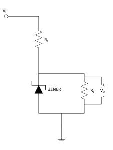
Figure 6.6 – Basic regulator circuit using Zener diode
