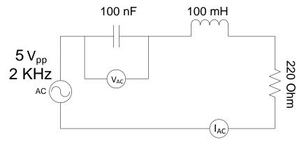
Figure 3.3 – Schematic for series RLC circuit
