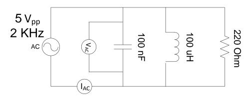
Figure 3.4 – Schematic for parallel RLC circuit
