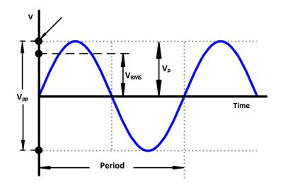
Figure 3 – Quantities of a sinusoidal signal
