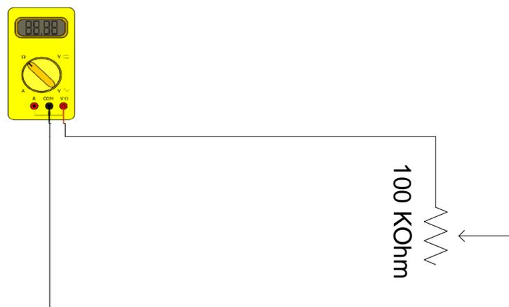
Figure 1.6 – Potentiometer experiment schematic
