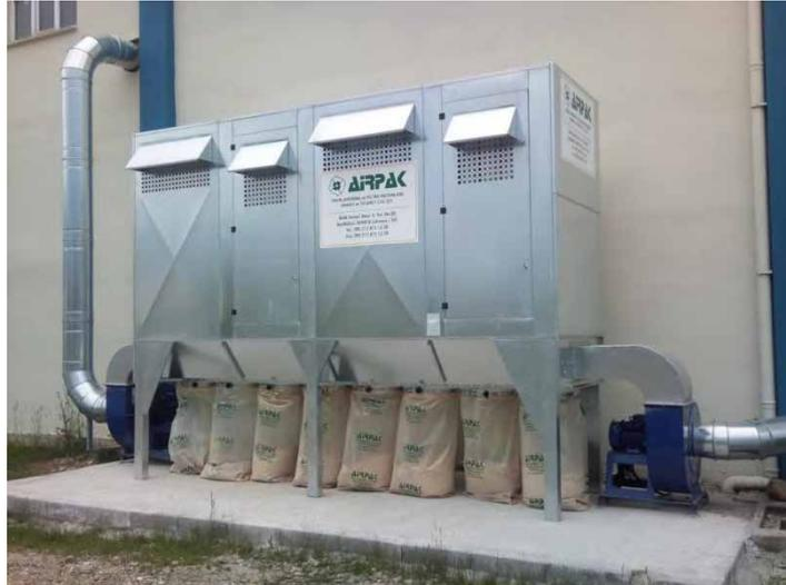
**Figure 3.** Bag Type Filter Dust Extraction System <sup>5</sup>
